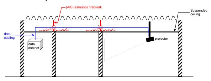
Example of damaged asbestos following installation of data cabling
